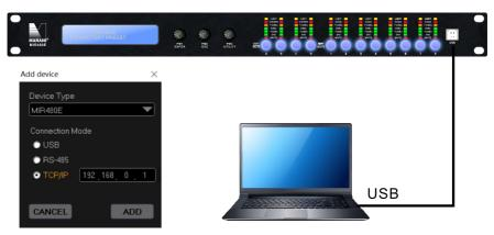
2. When using the network interface to connect, select on "Add New" window the TCP/IP interface, then use a Category 5/6 network cable to connect the ETHERNET port of the processor to the network adapter interface of the PC, and adjust the IPv4 address option in the corresponding network adapter in the Windows network settings to DHCP automatic acquisition, and then Open the software to automatically discover the current processor.
