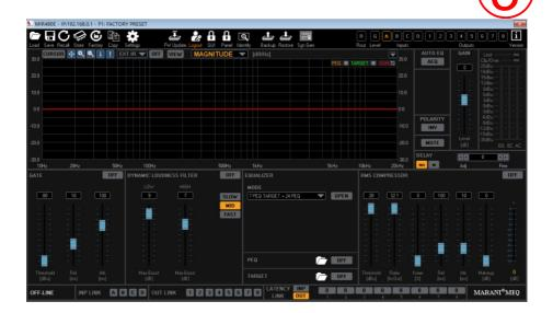
4. The administrator has the highest authority of the machine. After logging in to the administrator account, all or part of the output processing modules can be locked. The locked part can be hidden or not. The hidden output part is completely invisible in the non-administrator state. Admin Login
